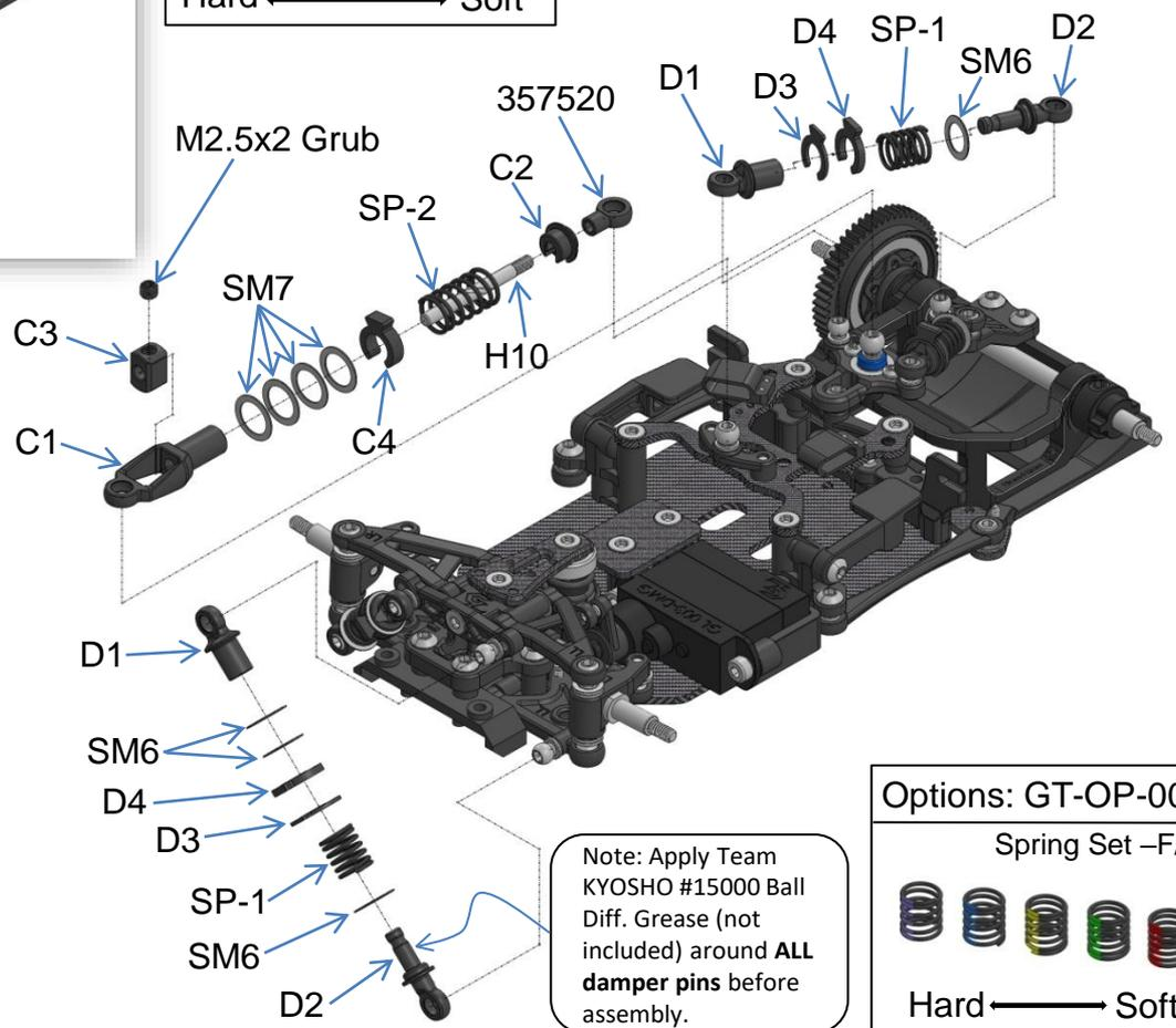
Note: Apply Team KYOSHO #15000 Ball Diff. Grease (not included) around **ALL** damper pins before assembly.
