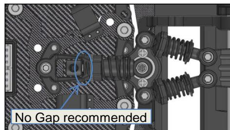
Adjust the C3 (page 19) with NO gap but need to keep the point 8 Front and Rear chassis in straight. This Gap = Down Stop for having unstable in all the time running on the high traction RCP track.
