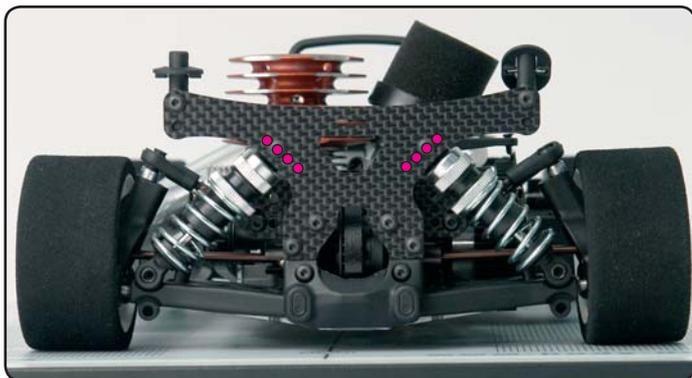
The upper and lower shock mounting positions determine how much leverage the lower suspension arm has on the shock when compressing it, and how progressive the suspension is. Different shock position settings change how the shock reacts to compression.
