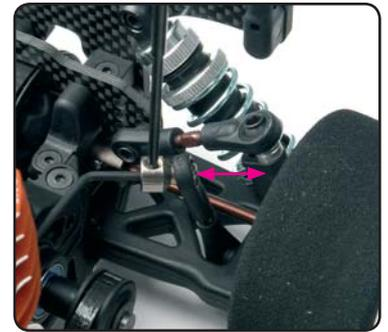
You may also adjust the rear anti-roll bar stiffness by using rear anti-roll bar wires of different thickness:
