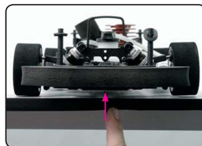
3. Adjust the preload on the REAR springs until both front wheels lift at the same time.
