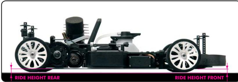
Ride height is the height of the chassis in relation to the surface it is sitting on, with the car ready to run. Ride height affects the car's traction since it alters the car's center of gravity and roll center. Because of changes in suspension geometry and ground clearance, there are negative consequences to altering ride height too much.
