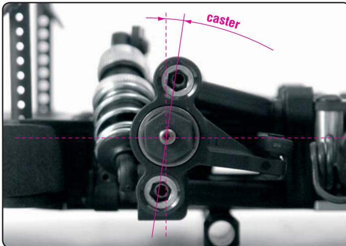
Caster describes the forward/backward angle of the front steering block with respect to a line perpendicular to the ground.
