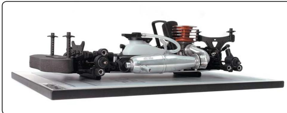
1. Place the droop gauge support blocks on the setup board, and then place the chassis on the support blocks. Make sure the chassis is solidly mounted on the support blocks so it does not move.
