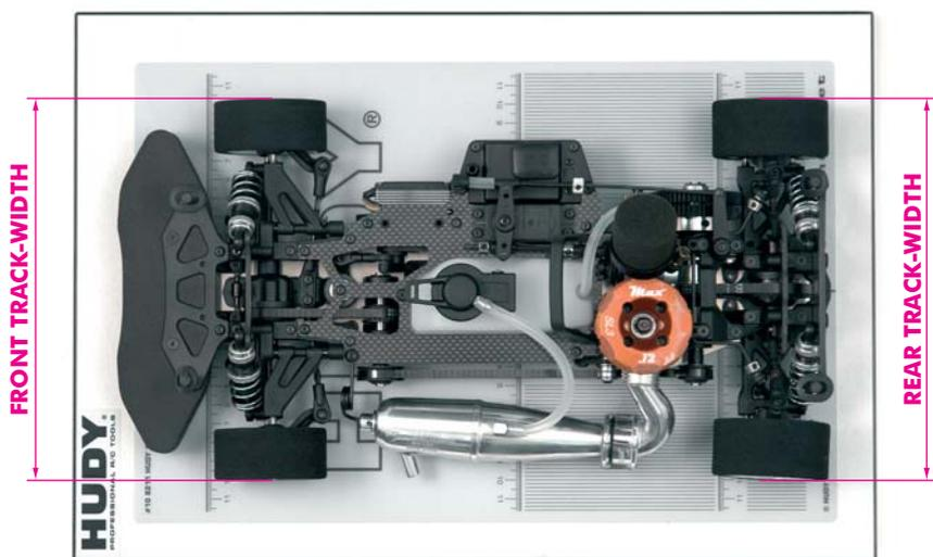
Track-width is the distance between the outside edges of the wheels, front or rear, and it affects the car's handling and steering response.
