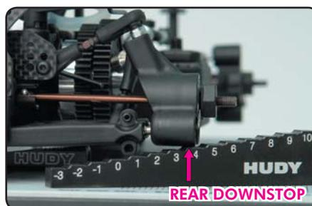
Downstops limit how far the suspension arms travel downward, which determines how far upward the chassis rises. This affects the car’s handling (due to effects on camber and roll-center) and the ability of the tires to “follow” the track. The effects may change with the type of track and/or amount of grip available.
