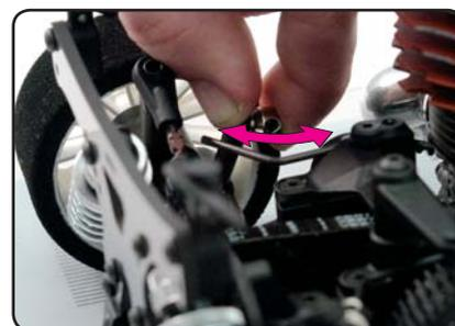
INCREASE the length of the rear anti-roll bar linkage diagonally across from the FRONT wheel that lifted first, and decrease the length of the other linkage. Adjust both linkages in equal but opposite directions.
