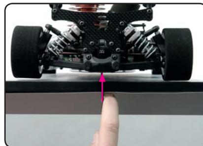
3. Adjust the preload on the FRONT springs until both rear wheels lift at the same time.
