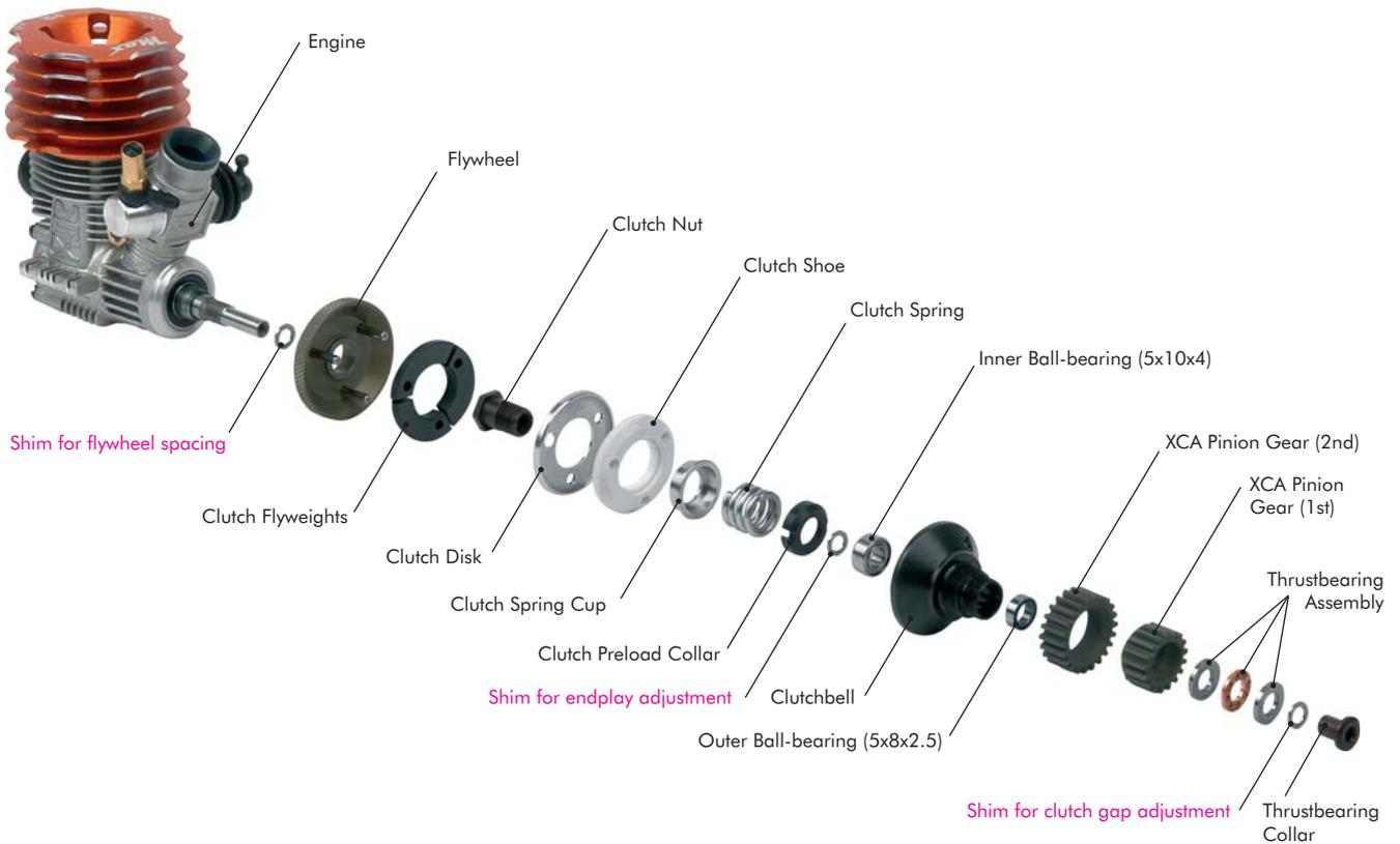
The XCA (XRAY Centrifugal-Axial) Clutch must be properly set up before driving the car the first time. A properly set up clutch will have a dramatic impact on the performance and drivability of the NT1.
