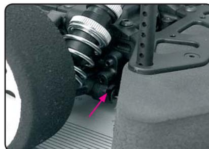
6. Loosen the lower setscrews in the left and right front anti-roll bar mounts. Adjust one or both eccentric cams until both rear wheels lift from at the same time. Re-tighten the setscrew(s) to secure the adjusting cam(s).
