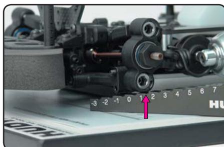
3. Using the droop gauge, measure the downstop value from the bottom of the front steering blocks / rear uprights..
